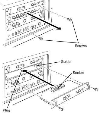
Figure shows HDB 15-PIN terminal (Optional parts).
