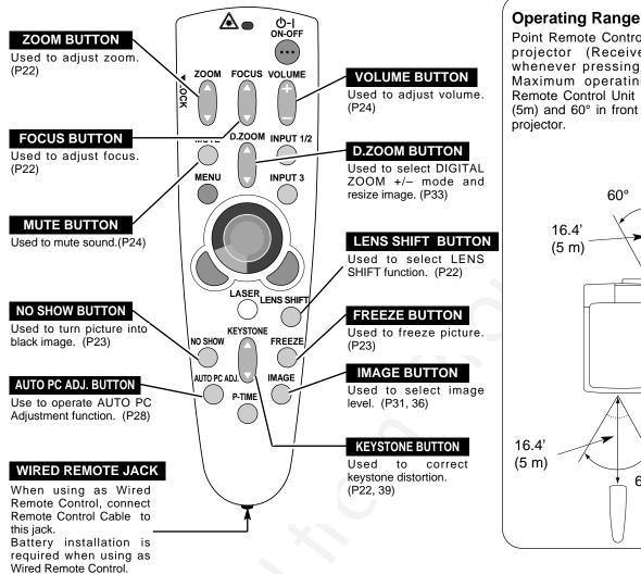
Point Remote Control Unit toward projector (Receiver Window) whenever pressing any button. Maximum operating range for Remote Control Unit is about 16.4' (5m) and 60° in front and rear of a
